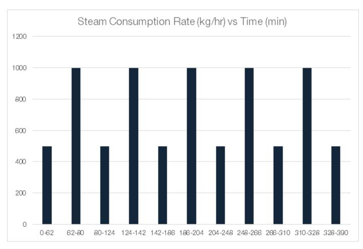
Plot 1: Steam Consumption (kg/hr) by the RTE/H System during a Shift
